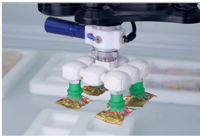
Bellows suction cups SPB2f when handling pouches
